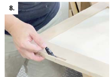
8. Install Clamex connectors; male half on the access panel
