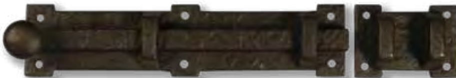
70-300 - Shutter Slide Bolt 6-1/2" x 1-1/2" Catch 2" x 1-1/2" Throw 2"
