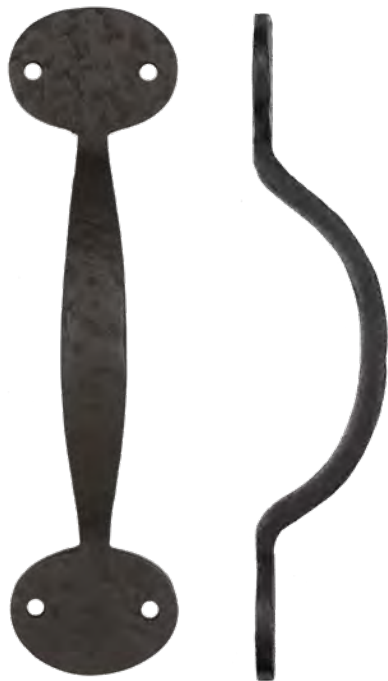
7-1/2" Pull Handle - Bean 40-105-B Dimensions: 7-1/2" L x 2" W Screw: 1" Round | #10 Stainless
