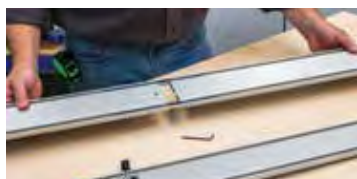
Aluminum guide rail leads cuts precisely along a straight line
