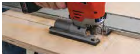
Aluminum guide rail leads cuts precisely along a straight line
