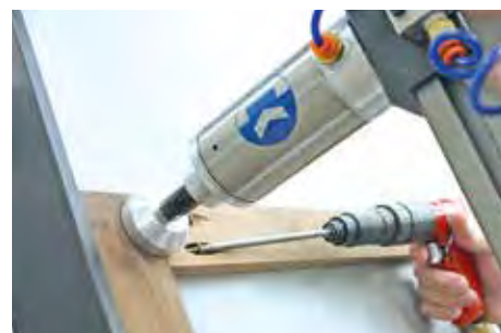
Flush Face Frames Made Easy: 1) Align stile and rail along squaring fence 2) Adjust clamp cylinder and secure joint line 3) Drive self-tapping screw
