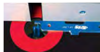
Step on the end of each setup bar precisely sets fence offset distances on the router table or table saw.
