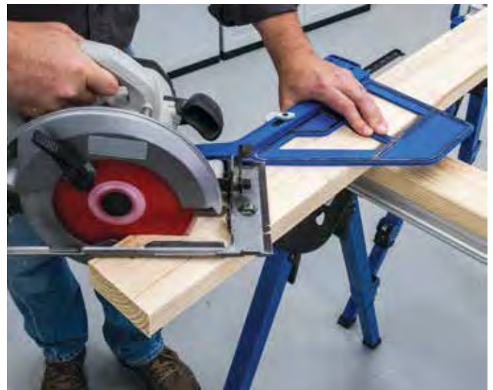
Cutline indicators show exactly where your saw will cut
