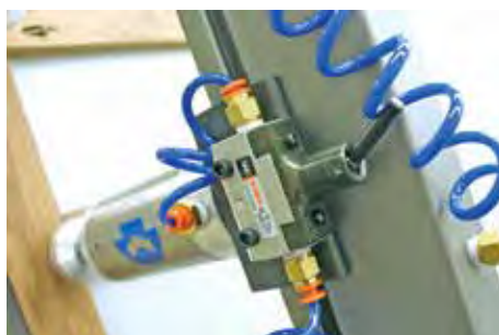
Flush Face Frames Made Easy: 1) Align stile and rail along squaring fence 2) Adjust clamp cylinder and secure joint line 3) Drive self-tapping screw
