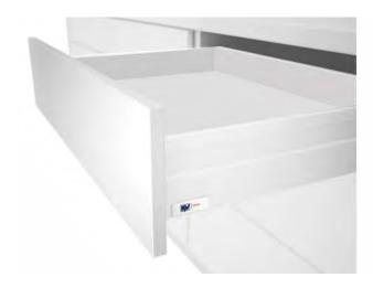
Alphabox offers style and configuation possibilities with contemporary side wall extensions. It features slim, molded side panels. Available with soft close, push-to-open and push-to-open/soft close drawer closure. Standard drawer height is 116mm/4.57" - greater drawer depth is possible by adding optional side rails\*\*\* or glass panels.\*\*\*
