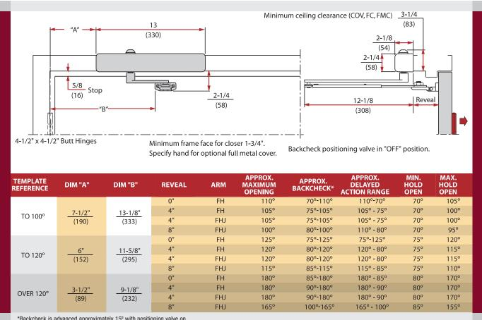
\*Backcheck is advanced approximately 15° with positioning valve on.
